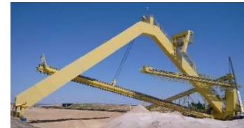
Combined Stacker / Reclaimer, Russalt, Russia, Span 75 m
