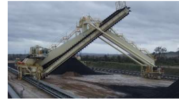
Reclaimer with double boom, Australia
