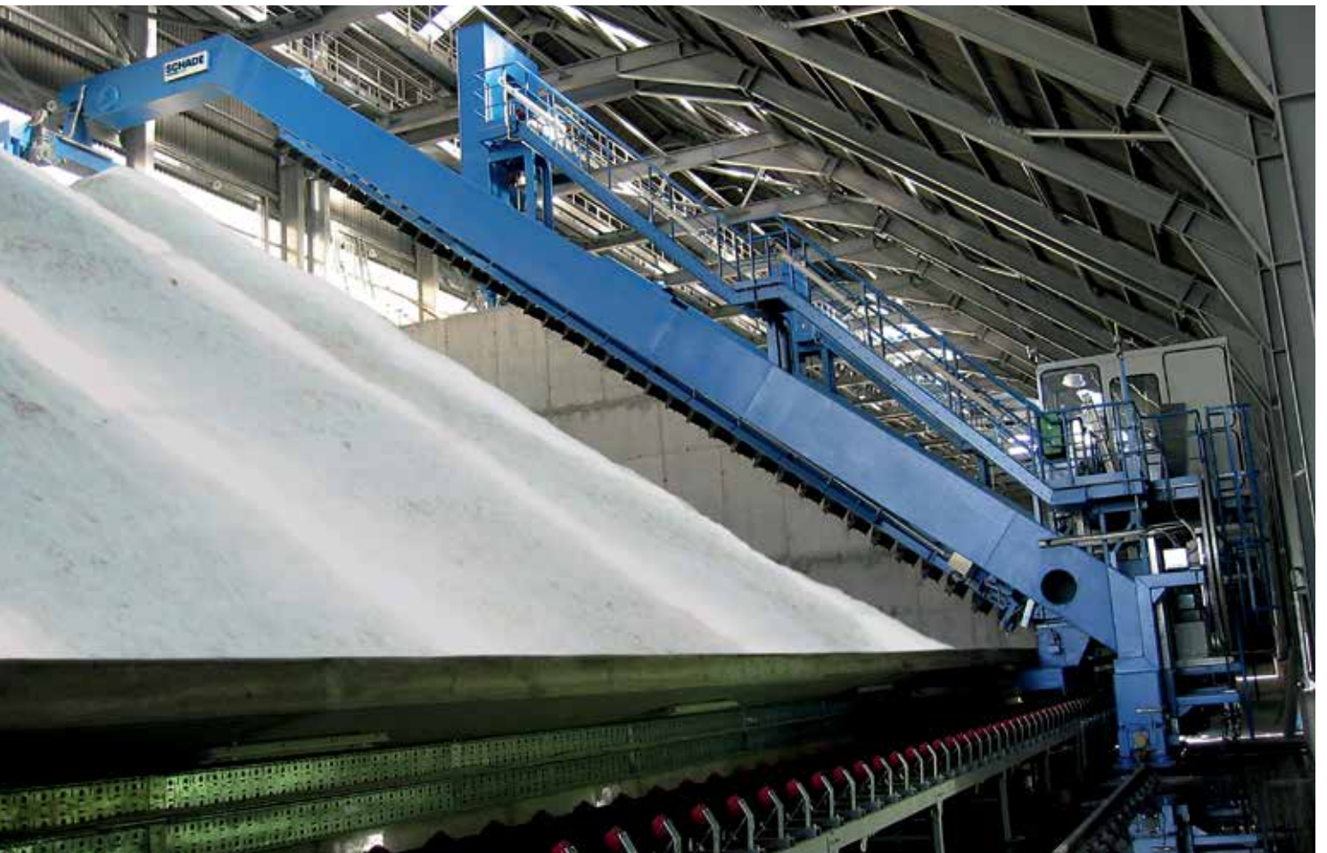
Semi-Portal Scraper Reclaimer, 21 m span, 150 t/h, additives
