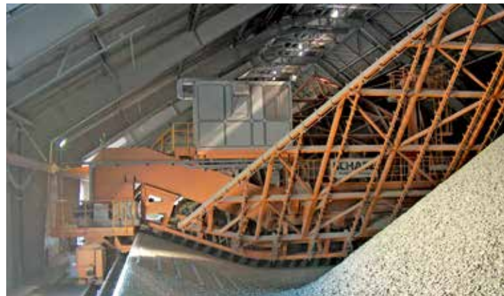
Bridge Scraper Reclaimer, 27.5 m span, 300 t/h, Gypsum
