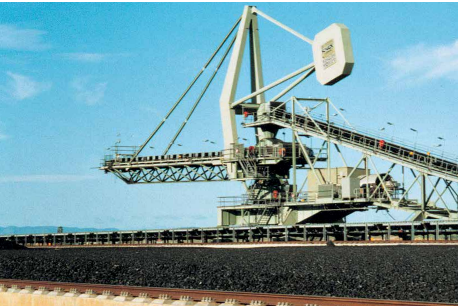
Fig. 1 Slewing/Luffing/Stacker for 2,750 t/h Coal
