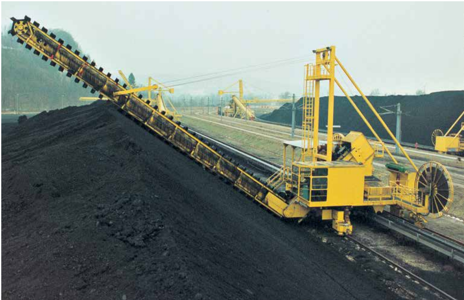
Cantilever Scraper Reclaimer designed for frozen Coal
