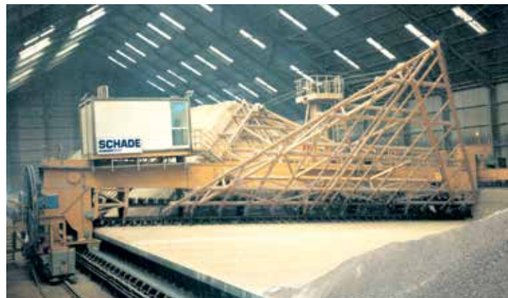
Bridge Scraper Reclaimer, 26.4 m span, 250 t/h, Limestone
