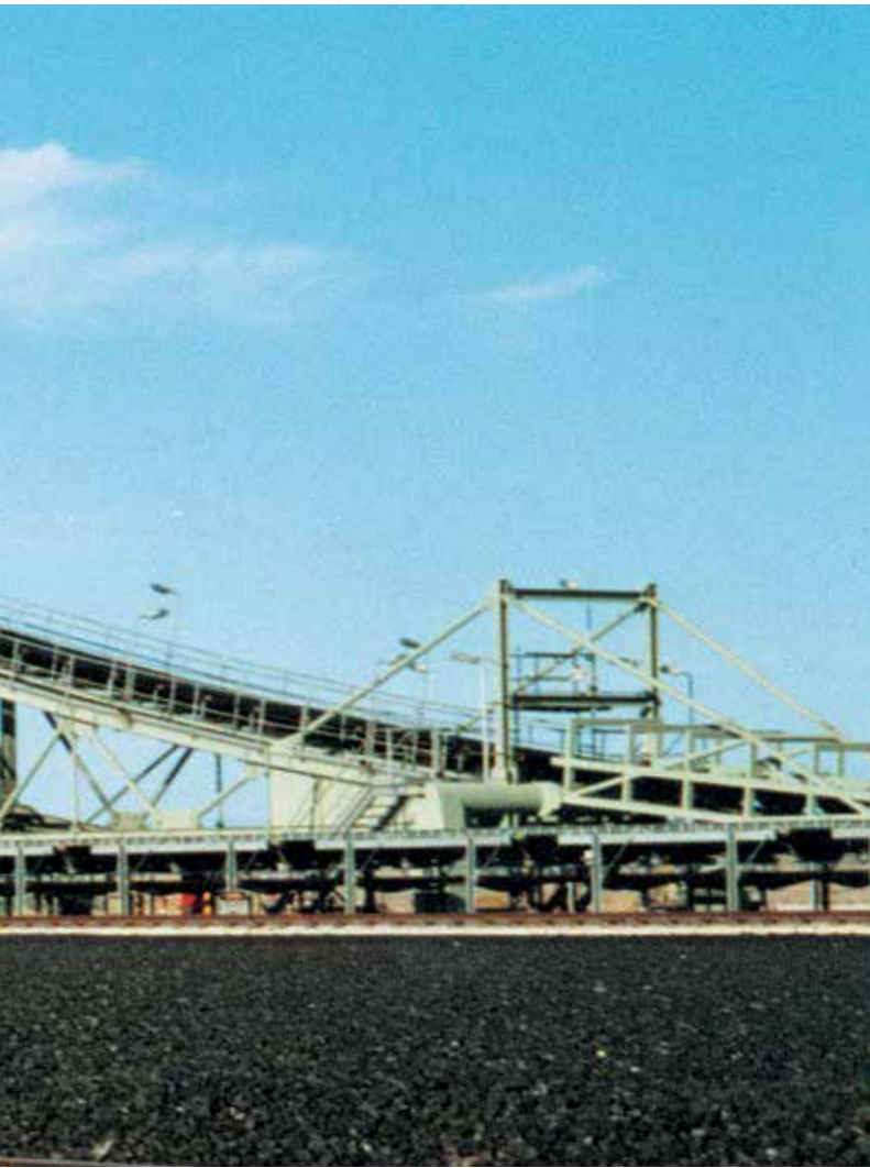
Fig. 2 Slewing/Luffing Stacker for 1,000 t/h Coal
