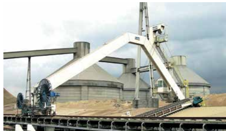
Portal Scraper Reclaimer, 33 m span, 600 t/h, Slag
