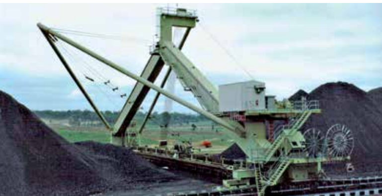
Portal Bridge Reclaimer, 50 m span, 600 t/h, Coal
