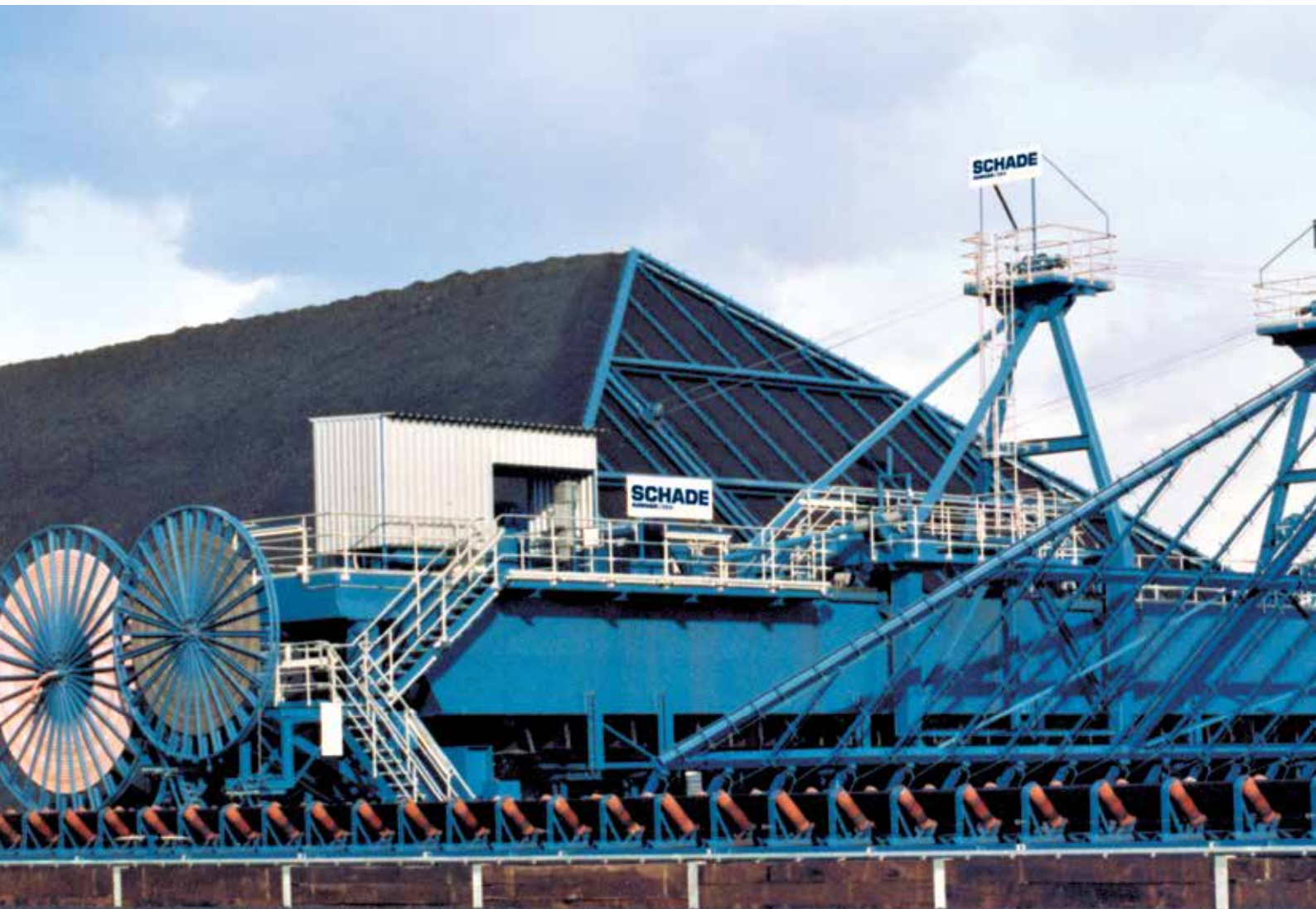
Bridge Scraper Reclaimer, 50 m span, 1,100 t/h, Coal
