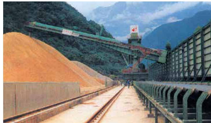
Fig. 3 Luffing Stacker for 2,000 t/h Limestone
