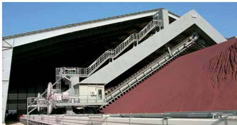
Portal Scraper Reclaimer, 49 m span, 550 t/h, additives
