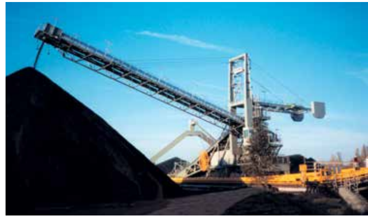
Fig. 2 Slewing/Luffing Stacker for 1,000 t/h Coal
