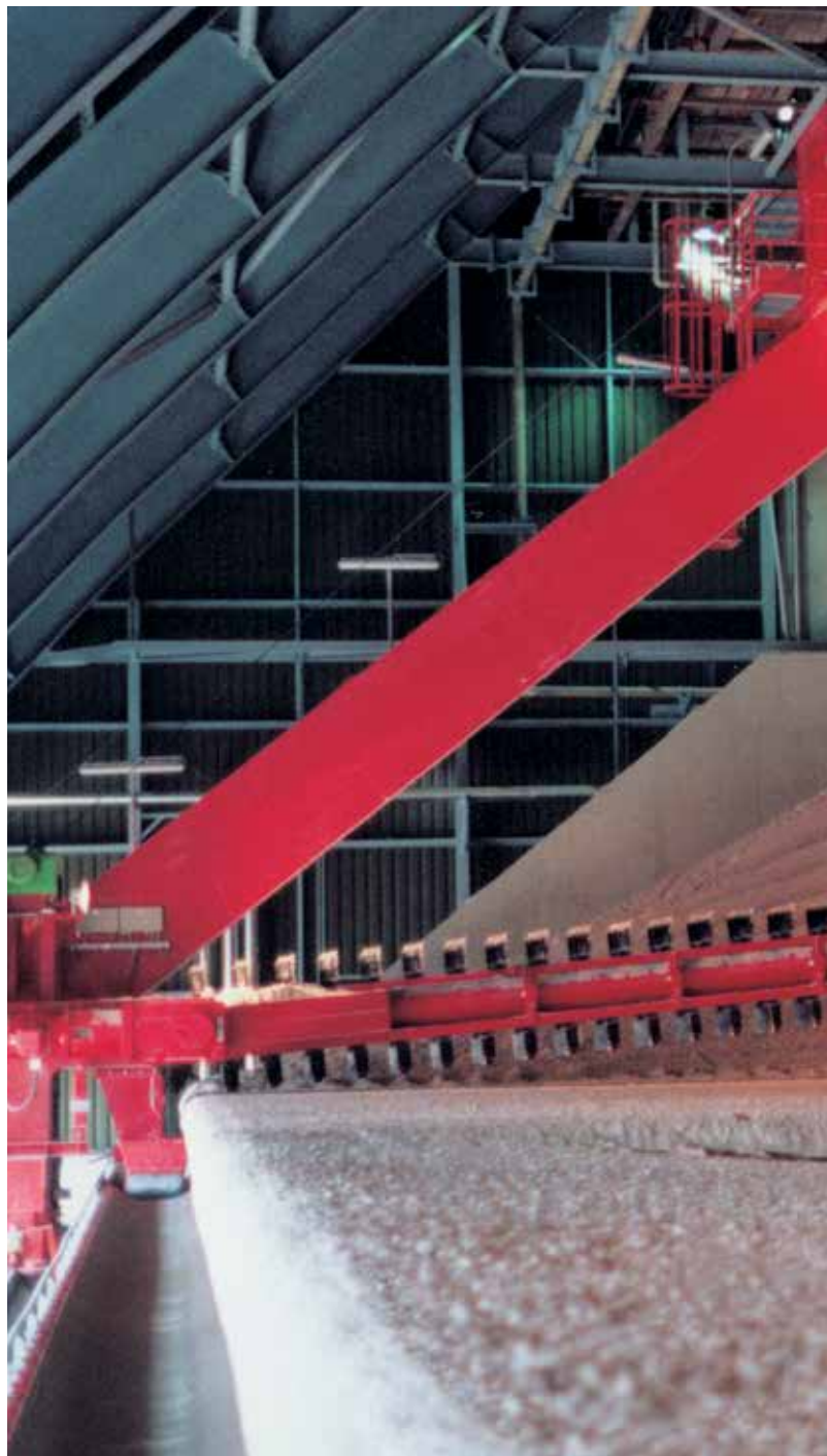
Portal Scraper Reclaimer, 32 m span, 400 t/h, FGD-Gypsum
