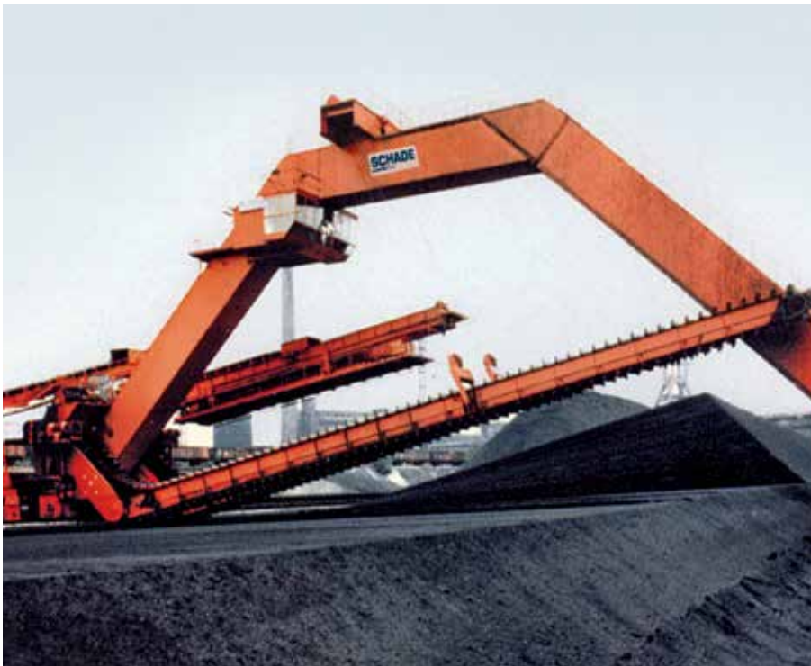
Combined Stacker Reclaimer, 47 m span, stacking 1,500 t/h, reclaiming 900 t/h, Coking Coal
