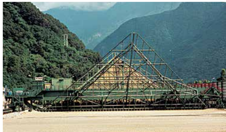
Bridge Scraper Reclaimer, 56 m span, 1.200 t/h, Limestone
