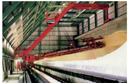
Semi-Portal Scraper Reclaimer, 14 m span, 80 t/h, FGD-Gypsum
