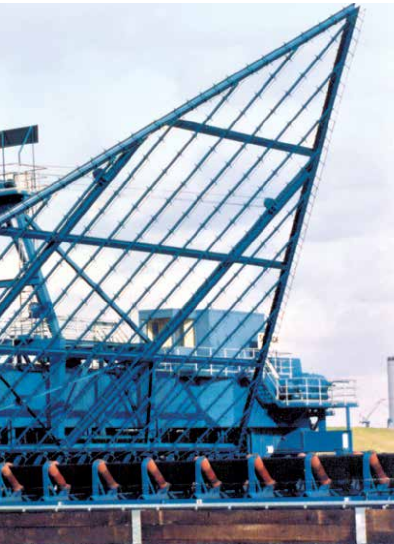
Bridge Scraper Reclaimer, 26.4 m span, 250 t/h, Limestone
