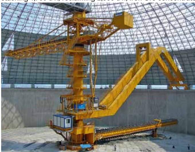
Circular Stacker / Semiportal Scraper Reclaimer, dia 120 m, stacking 3,000 t/h, reclaiming 1,500 t/h, Coal
