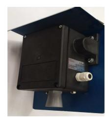
The COU-ET presence sensor is designed to detect people and objects within the range of the ultrasonic sensor detector. It is suitable for measuring the filling level of tanks with the setting of alarm thresholds. The COU-ET presence sensor meets the requirements for explosion-proof devices and can be used as a group I device in category M1 and group II in categories 1G and 1D.
