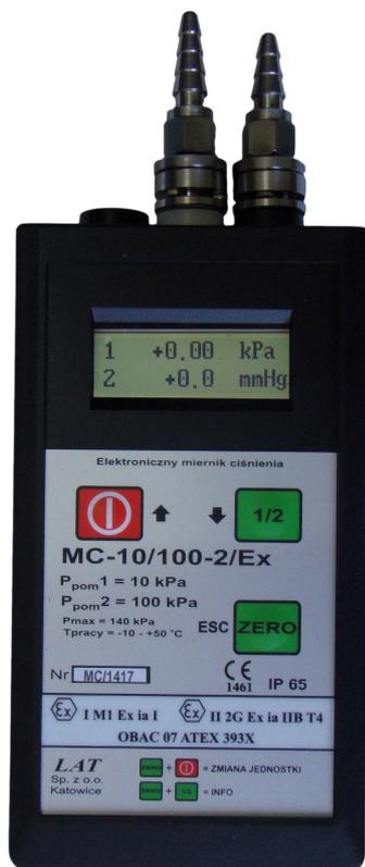
The MC-10/100-2/Ex pressure meters are electronic devices equipped in two pressure converters, one for differential pressure with  $\pm 10$  kPa measuring range, and another for relative pressure with  $\pm 100$  kPa measuring range.
