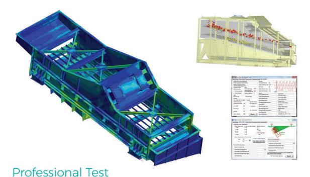
Each machine is tested using a vibration analyzer to find any dynamic irregulates in a vibrating screen. This information makes it possible to monitor the orbit diagrams, amplitude and frequency of vibration and FFT analysis. The integrated FFT analysis separates and analyzes frequency patterns that indicate possible mechanical problems.
