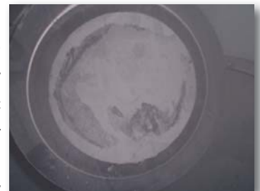
UCC TITAN HP seat shows little wear after a year in service
