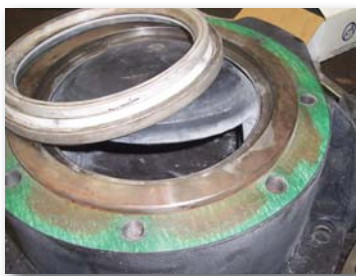
Worn inflatable seal required valve to be pulled out of service
